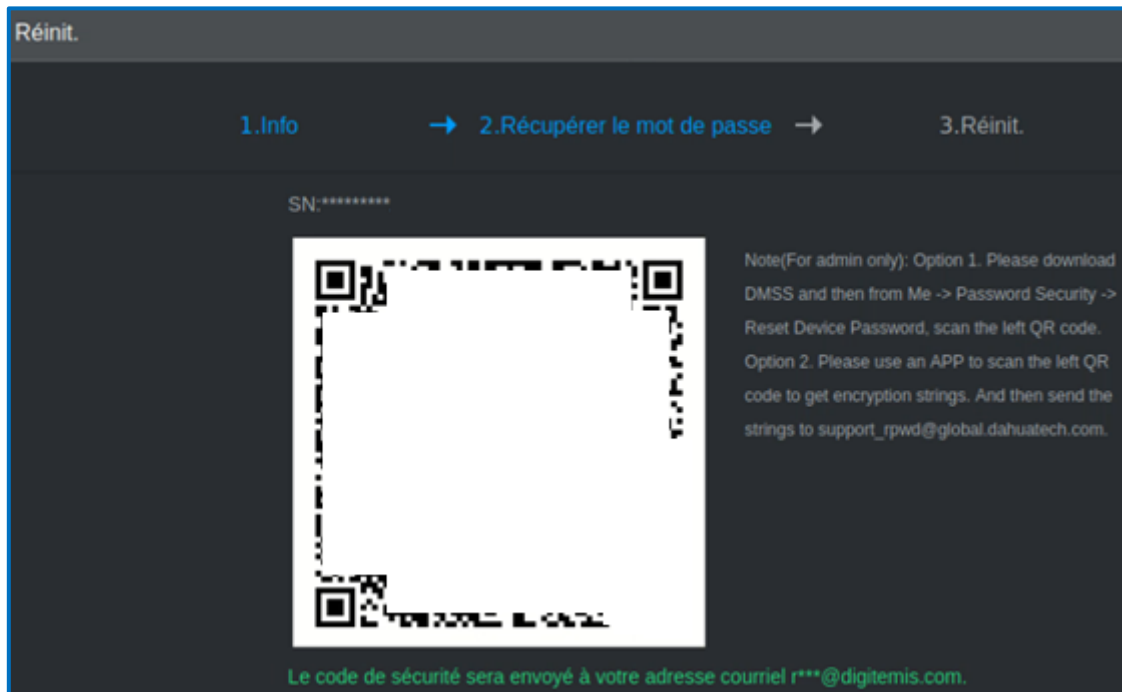
Figure 12 - Procedure for resetting the password of the "admin" account of the video recorder
